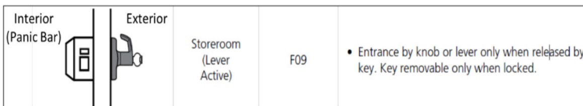
Figure 1 – Equipment Room Door Lockset Functionality
