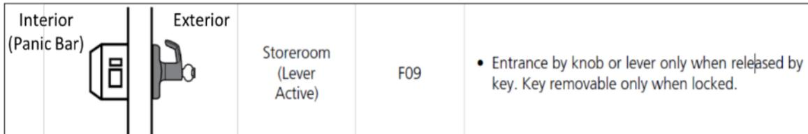
**Figure 4—Equipment Room Door Lockset Functionality**
