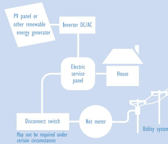
*This illustration shows a small electricity generation system's major components and its connections to Rocky Mountain Power's system.*
