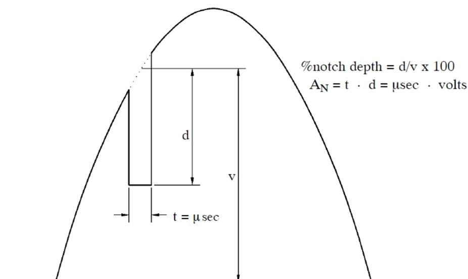
**Figure 1—Definition of Notch Depth and Notch Area**
