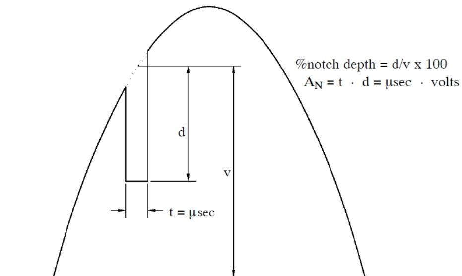
**Figure I—Definition of Notch Depth and Notch Area**
