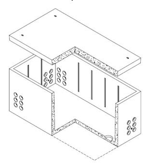
Figure I — 7' × 12' (94" × 155") Shallow Vault, Cutaway View
