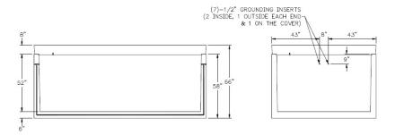
Figure 3— 7' × 12' (94" × 155") Shallow Vault Ground Grid Layout
