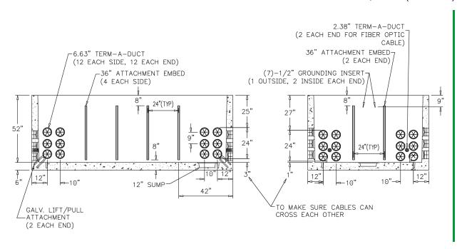
Figure 2— 7' × 12' (94" × 155") Shallow Vault Enclosure Layout
