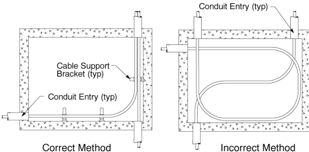
**Figure 9—Enclosure Cable Training and Support**
