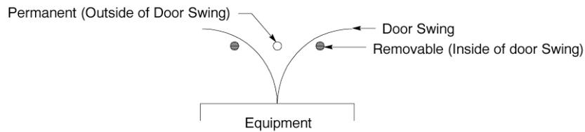
**Figure 12—Equipment Door and Barrier Post Positioning Detail**
