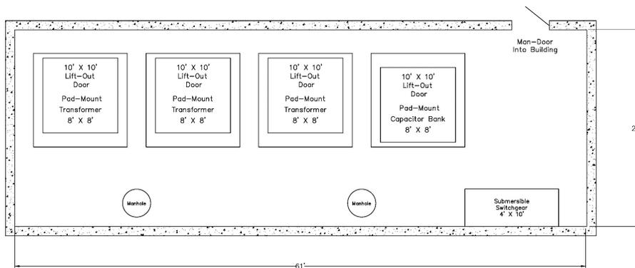
**Figure 5—Example of Underground 3-Transformer Vault with Capacitor Bank and Switch**
