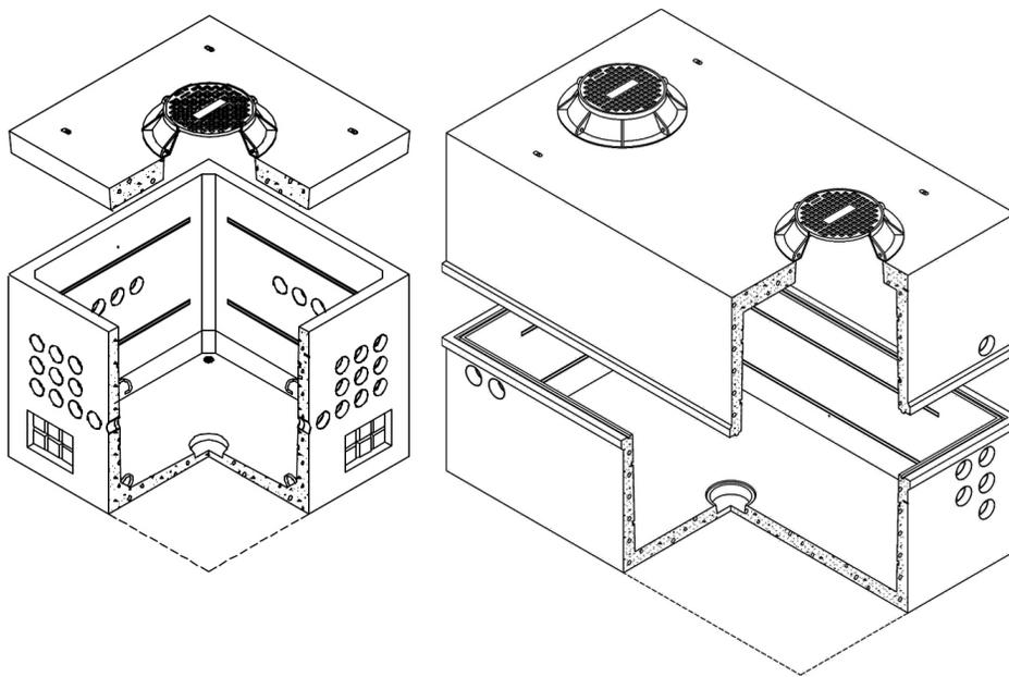
**Figure 4—Typical Manholes**
